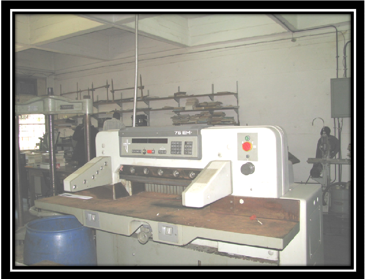
Figure 7: Old model guillotine machine in the Bindery Unit
