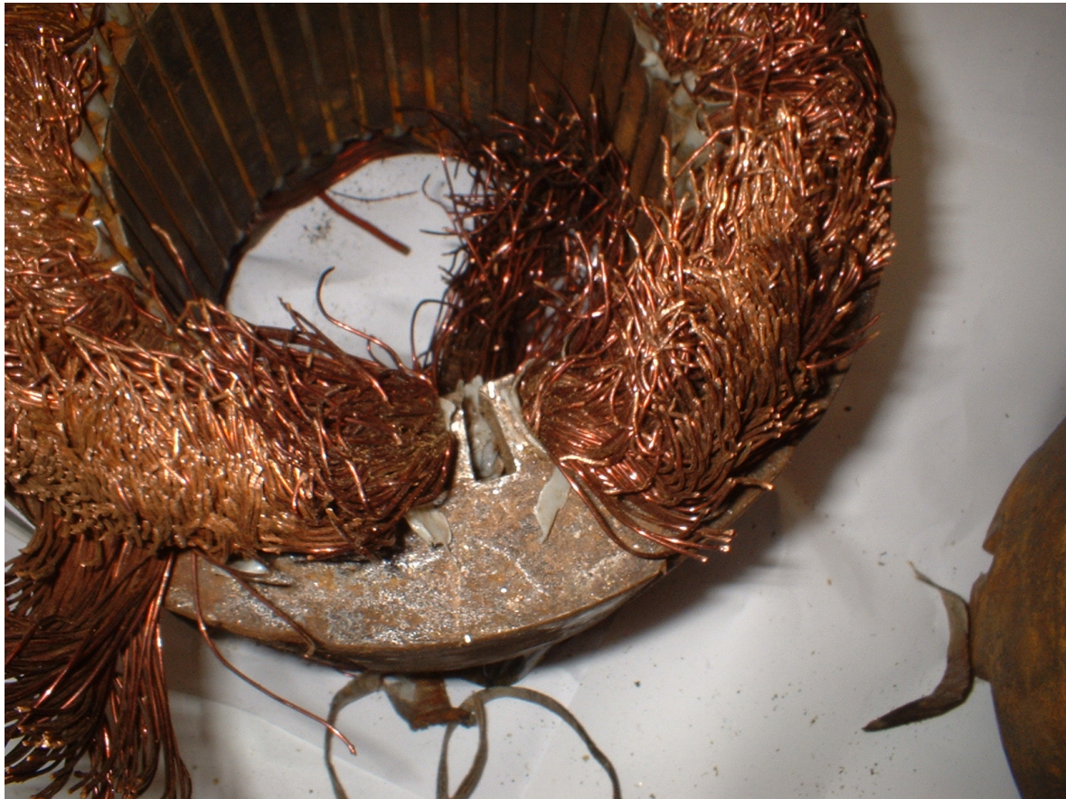
Figure 1-7 Stator Core showing a typical Stator Slot (Courtesy of UTH Workshop)
