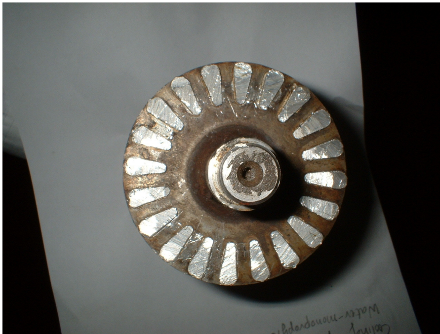
Figure 1-4 Cut away View of the Squirrel-Cage Class B Rotor for Induction Motor showing imbedded Aluminium Rotor Segments (Courtesy of UTH maintenance workshop)
