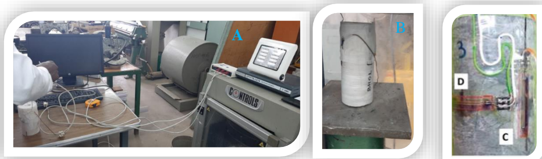
Figure 3.5 (A) setting up of an experiment, (B) Placing the sample on the platens of the testing chamber, connecting strain gauges to the core sample (C-Axial strain gauge and D-Radial strain gauge)
