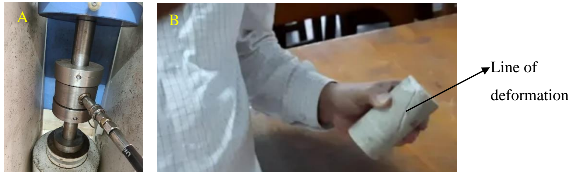
Figure 3.6. (A) Hoek Cell containing core sample undergoing triaxial compressive test process (B) Deformed core sample after the test
