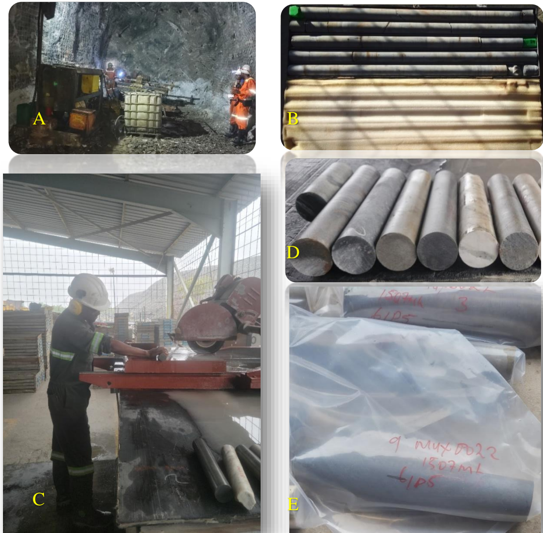
Figure 3.3 Showing (A) Core being drilled at an underground diamond drilling site, (B) Core samples packed for transportation, (C) Core samples being cut to 14 cm long size, (D) NQ size core samples and (E) Core samples packed in plastics for laboratory analysis
