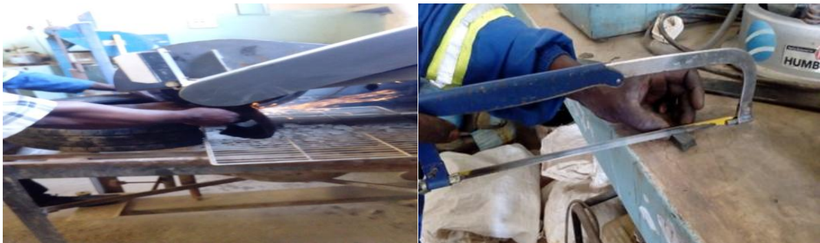
Figure 3.1: Process used to produce rubber aggregates from used tyres
