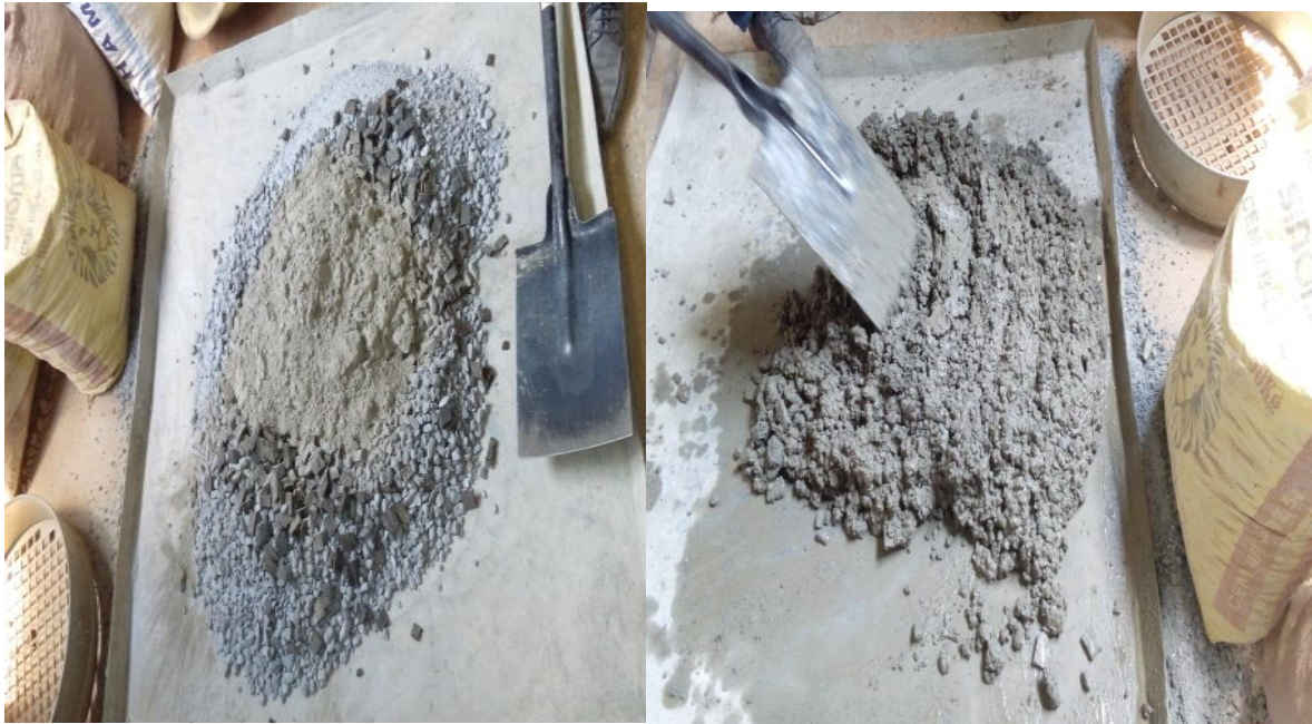
Figure 3.7: Preparation and mixing of concrete specimens (15% Rubber)
