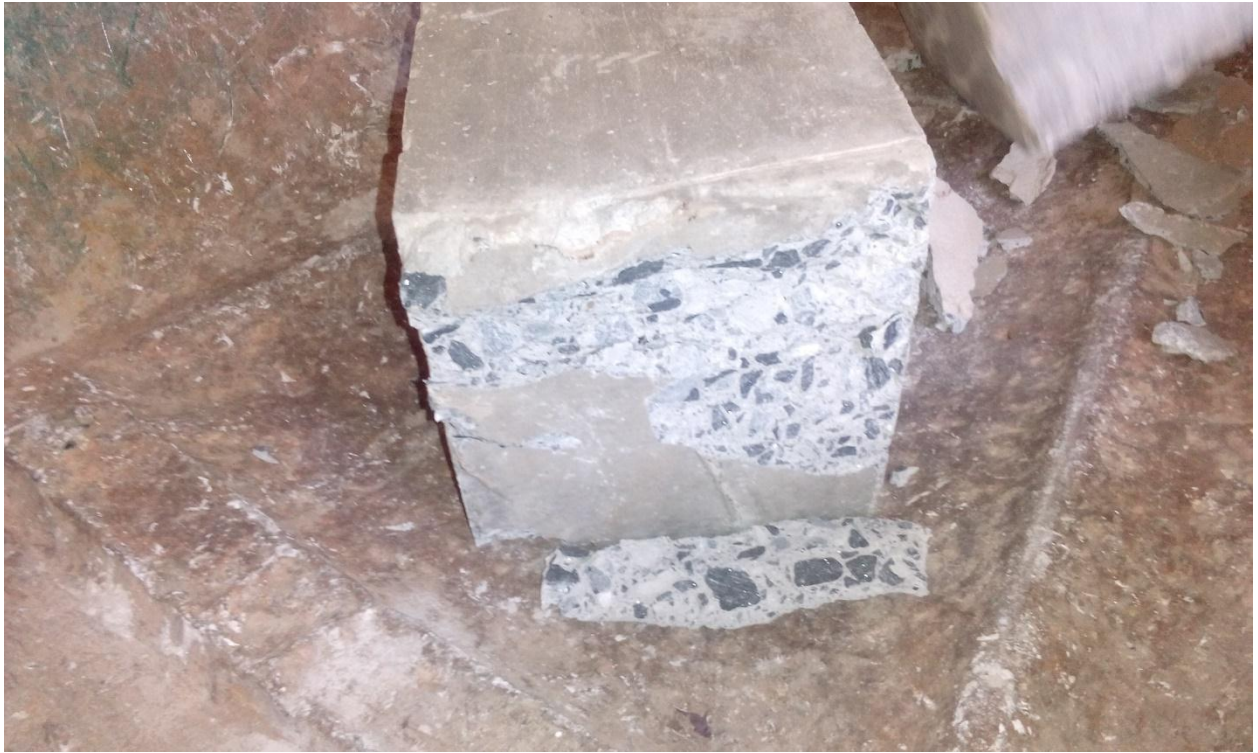
Figure E.5: Failure pattern of heated rubber reinforced concrete after being subjected to compression forces
