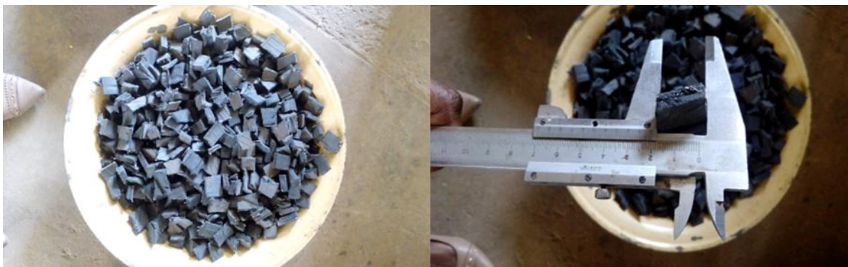
Figure 3.2: Coarse rubber aggregates obtained from used tyres
