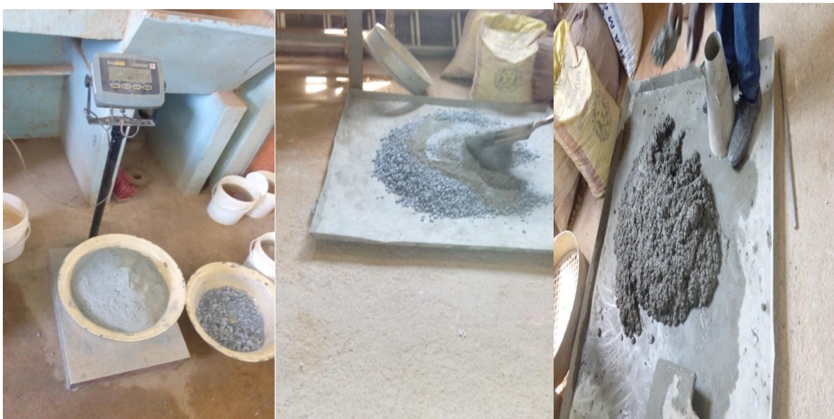
Figure 3.6: Preparation and mixing of concrete specimens (0 % Rubber)
