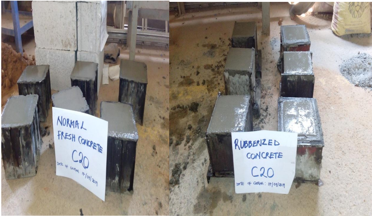
Figure 3.8: Casting of the control concrete and rubberized concrete specimens
