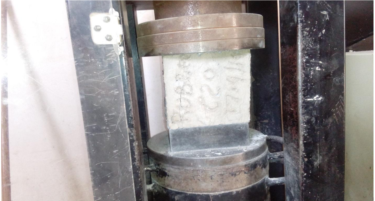
Figure E.3: Compression test of heated rubber reinforced concrete
