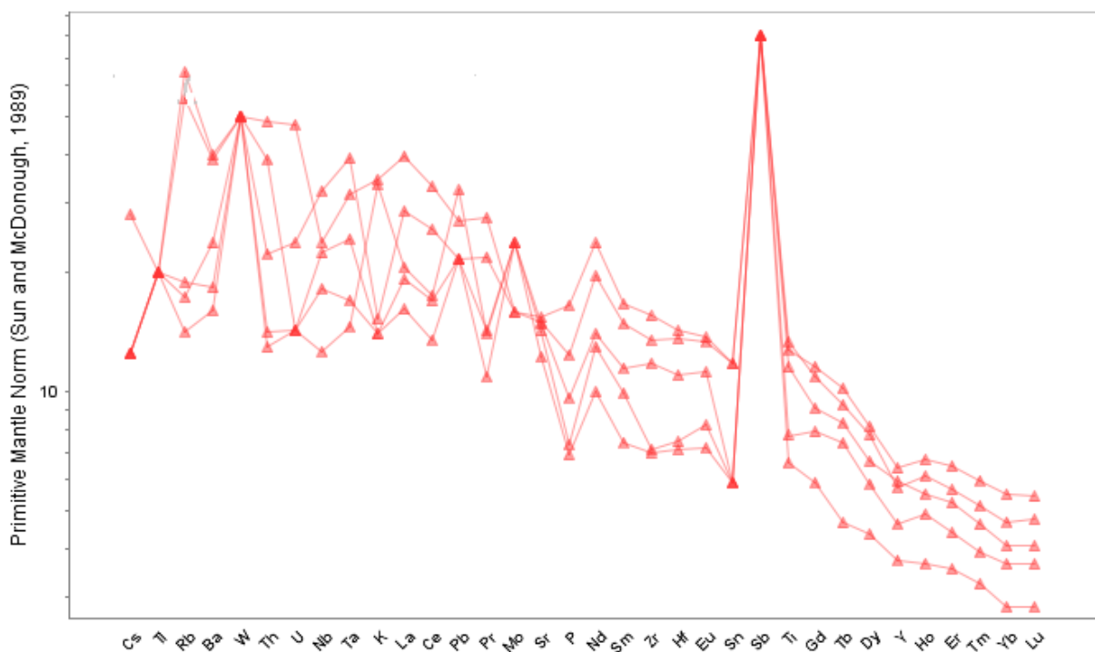
Figure 4.43: Primitive mantle-normalised multi-element spider diagram plot for the tholeiitic rock samples of the Study area, after Sun and McDonough (1989).
