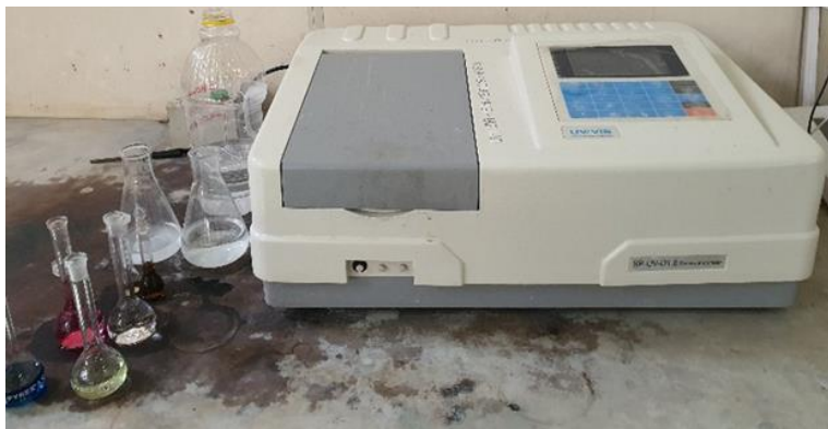
Figure 8: The SP-UV-D1.8 Spectrophotometer for the laboratory testing of phosphate, sulphate, sodium, potassium and nitrate.
