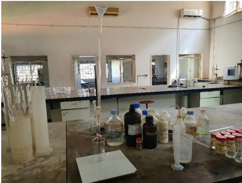
Figure 9: Titrimetric analysis using the volumetric method for the laboratory testing of chloride, calcium and total hardness.
