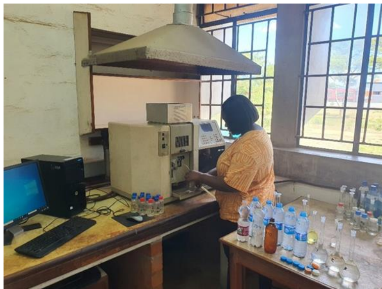
Figure 10: Laboratory testing of manganese, iron and lead using the Varian 55 Atomic Absorption Spectrophotometer.
