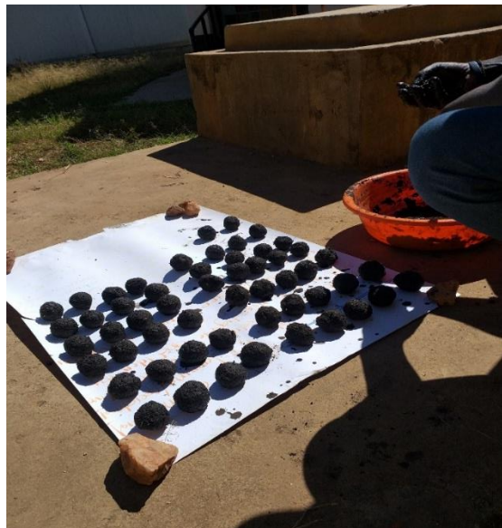
Figure 6: faecal sludge briquettes, drying in the sun.
