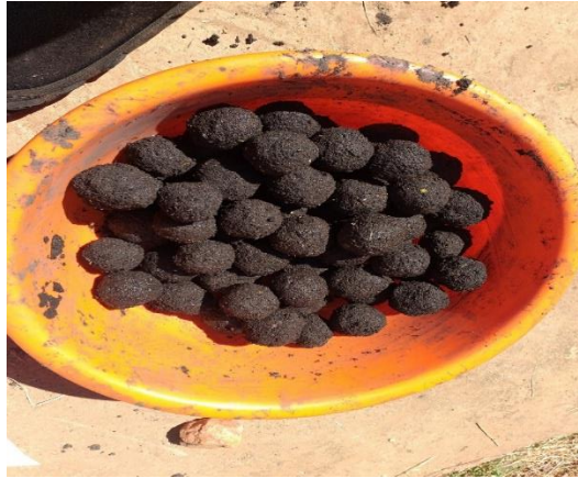
Figure 5: Hand moulded faecal sludge briquettes
