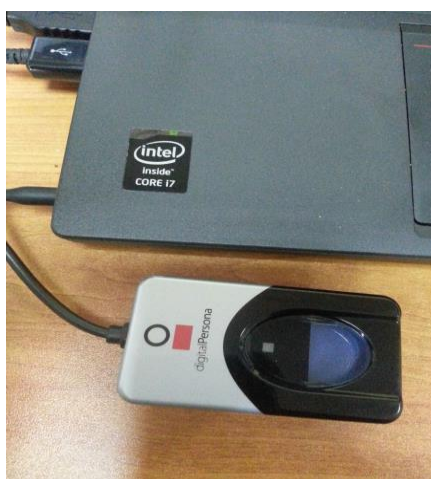
Figure 8: Laptop and DigitalPersonaU4500 fingerprint scanner used for this research
