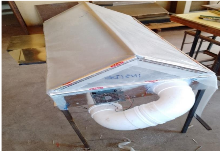
Figure 3.4b: Side view of the solar tunnel dryer with air recirculation path.
