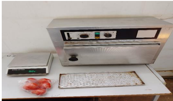
Figure 3.17: Apparatus for determining the moisture content of tomatoes.
