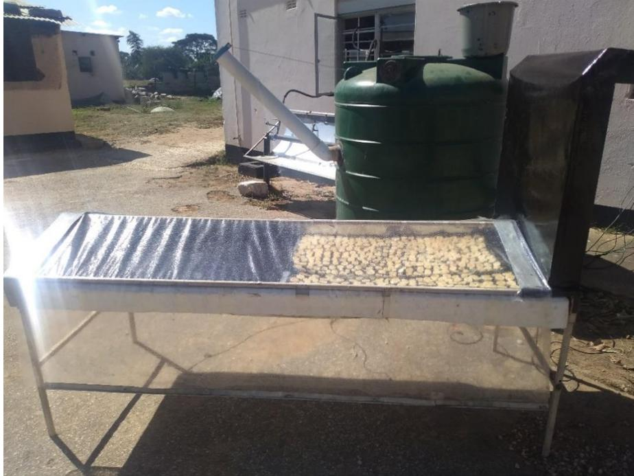
Figure 3-3 Solar tunnel dryer loaded with the sliced bananas
