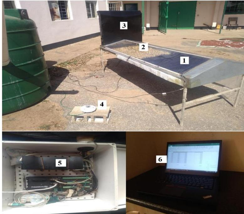
Figure 3-2 Experimental set-up of the solar tunnel dryer and the equipment (1) Collector unit, (2) Drying unit, (3) Bare flat-plate chimney unit, (4) Solar pyranometer, (5) Data logger, (6) Computer.
