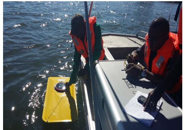
Figure 4- 5: Discharge measurements at Namwala
