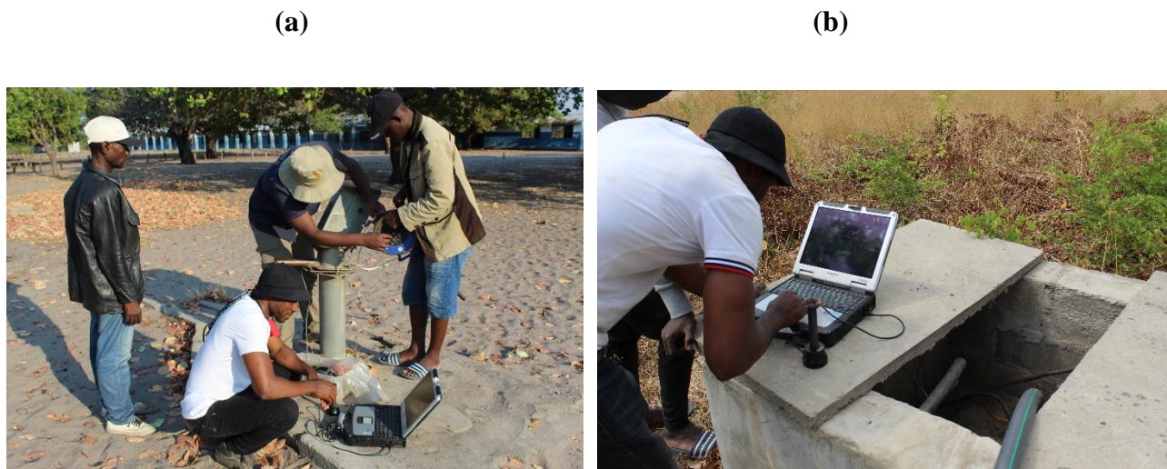
Figure 12. Field measurements of groundwater levels (a) Senanga (b) Lukulu
