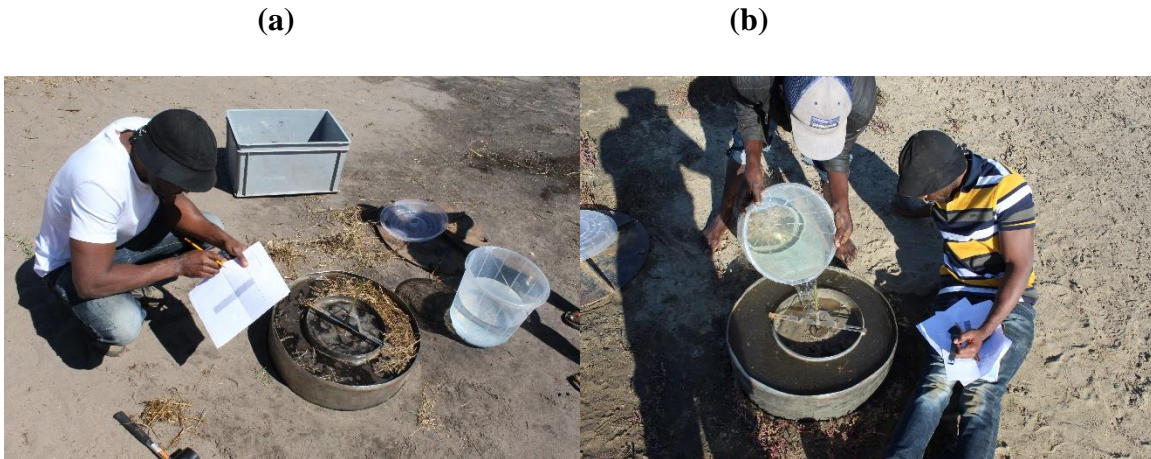
Figure 13. Field measurements of rate of infiltration at (a) Lukulu (b) Senanga
